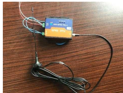
Figure 21, DTU & its Antenna
