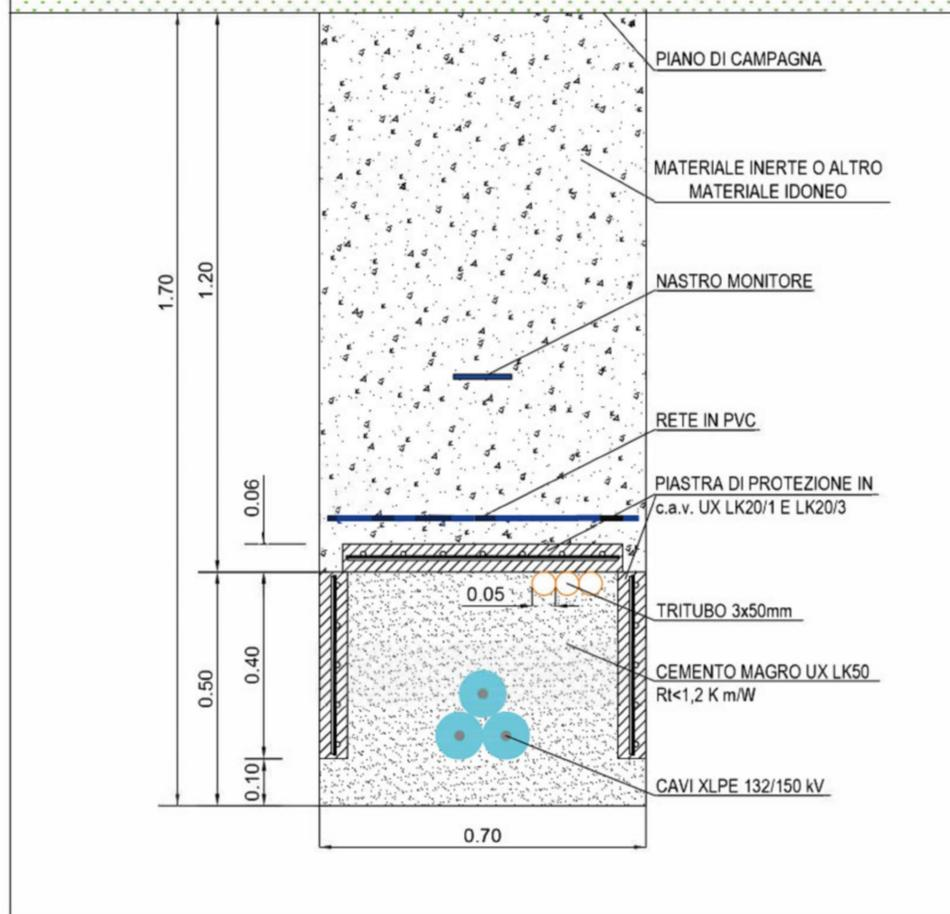
**SEZIONE TIPO - N°1 TERNA AT 132/150 kV**
