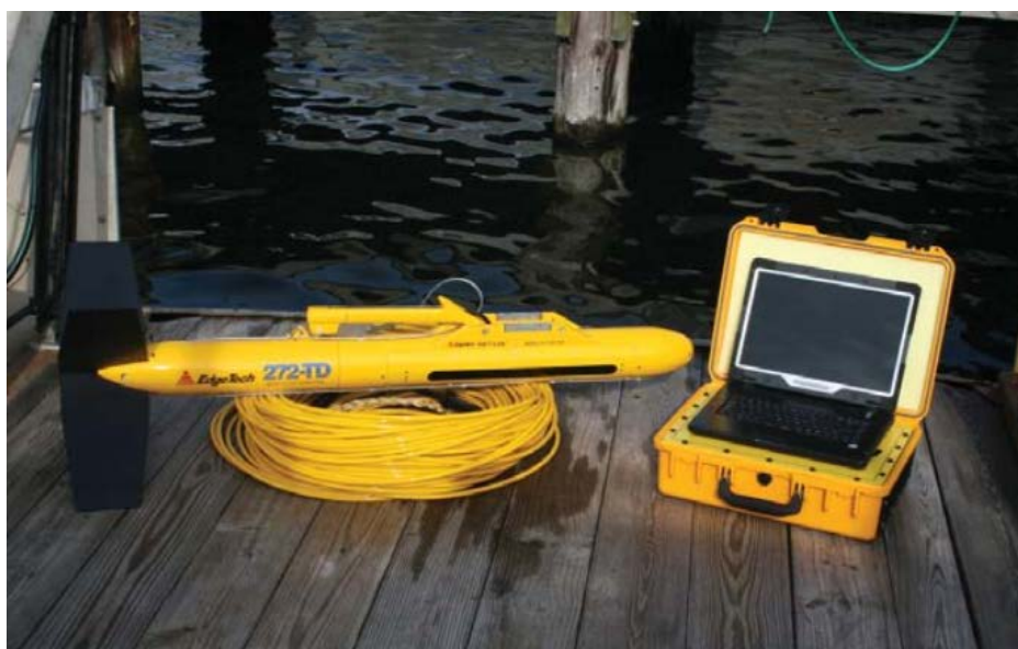
Fig.2: Side Scan Sonar Edge Tech 4100 - Modello 272TD Towfish
