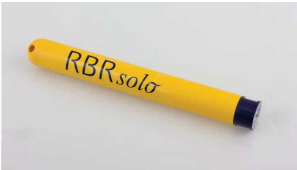
Fig. 2.6 - RBR “solo” pressure gauge (diameter = 2.54 cm, length = 22 cm) positioned on the seabed about 38 m away from briccola 121
