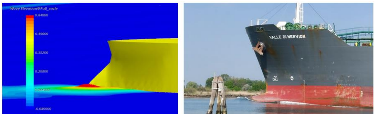
Figure 14: computed and experimental wave elevation near the bow
