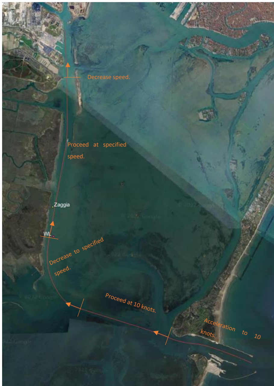
Figure 2.30. Vessel speed profile of in-bound passage.
