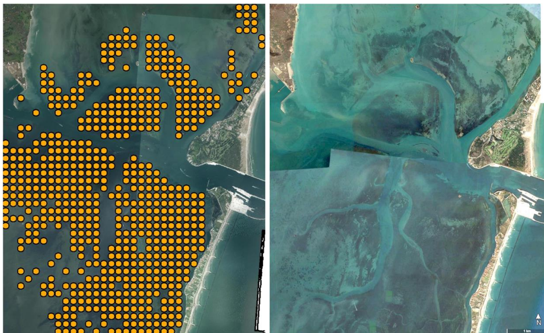
Figure 4 – Detail of the distribution of sea grass in the Malamocco basin, close to the inlet. On the left the grid adopted after controlling the GIS layer furnished by the Port Authority with the aerial photo of Google Earth (March, 2021) on the right. The grid is 200x200 m.
