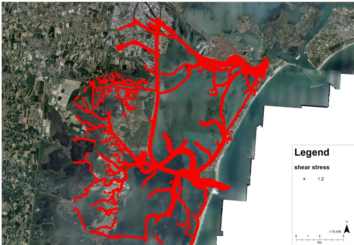
Figure 2 – The channel system of the Malamocco basin, where it has been assigned a critical shear stress of sediment of 1.2 Pa. The grid is 50x50 m.
