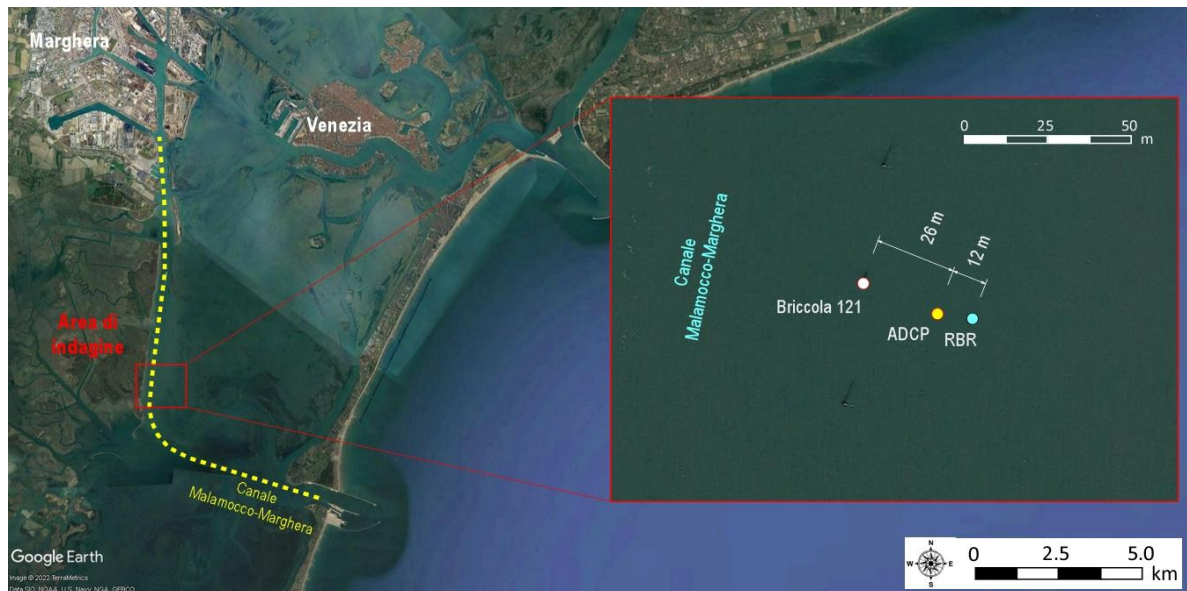
Fig. 2.1 - Survey area and instruments array (May 16 th campaign)
