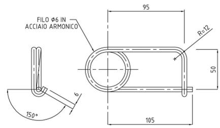
DETAIL SPILLONE PER PARAPETTO REMOVIBILE (SCALA 1:2)
