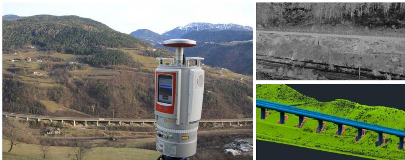
**Figura 2 – Rilievi Laser Scanner**
