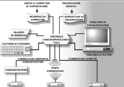
SCHEMA A BLOCCHI DEL SISTEMA ANTISTRUZIONE
