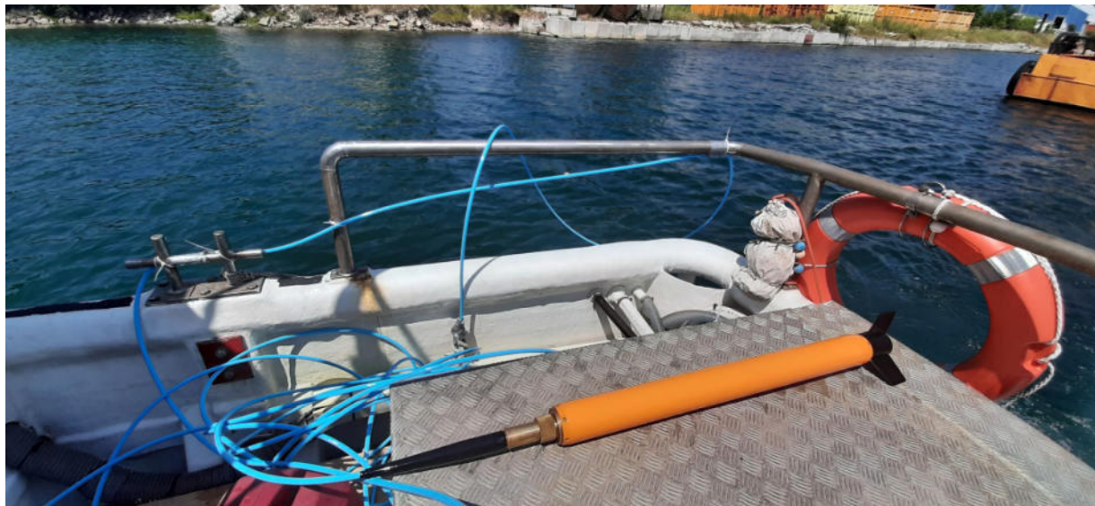
Foto - Magnetometro marino Explorer Marine Magnetics
