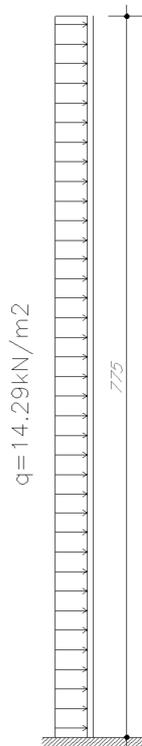
$$V = 14.29 \text{ kN/m}^2 * 7.75 \text{ m} = 110.7 \text{ kN/m}$$
