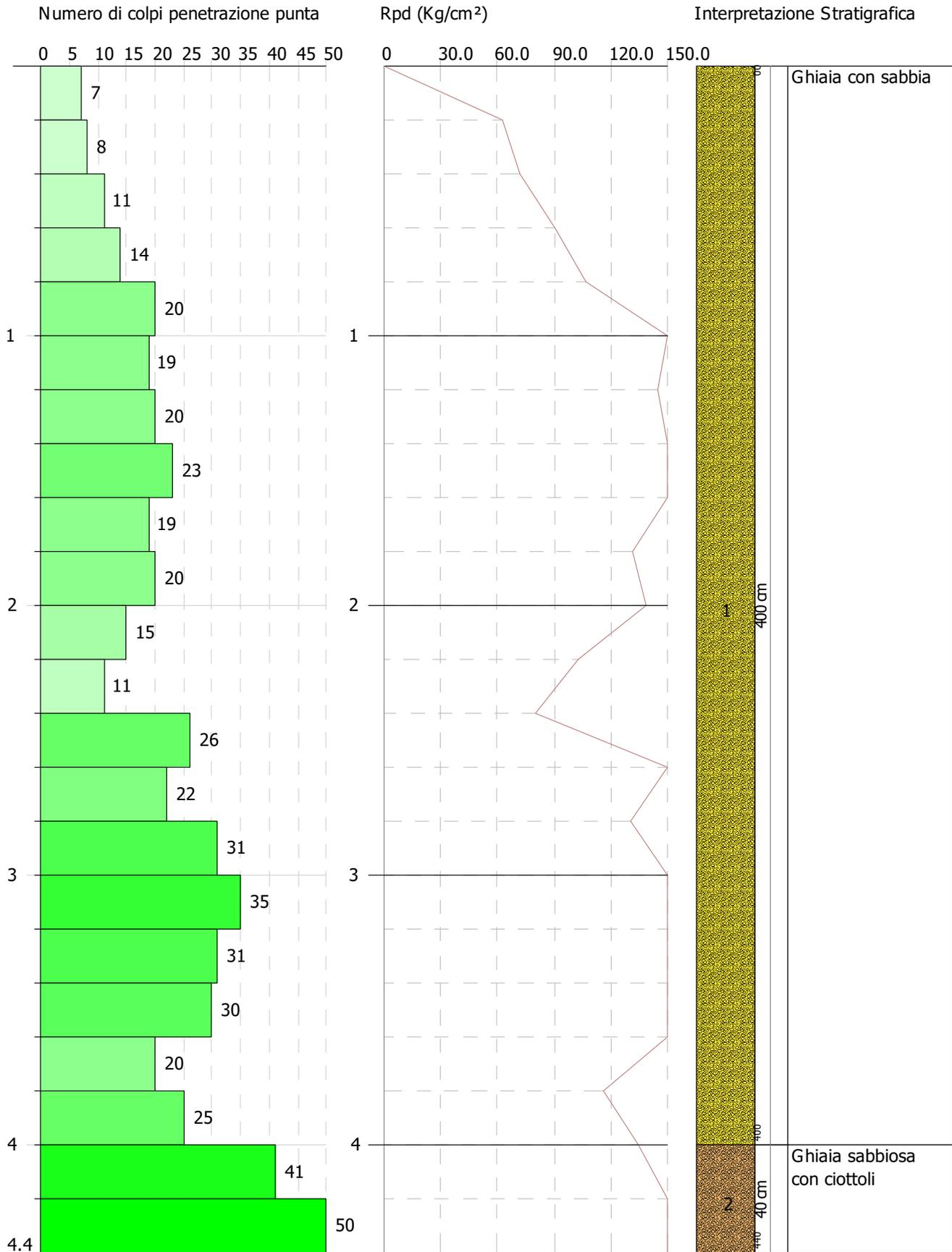
PROVA PENETROMETRICA DINAMICA DPSH6
