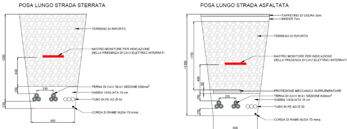
FIGURA 18: TIPOLOGICO POSA LINEE DI CONNESSIONE
