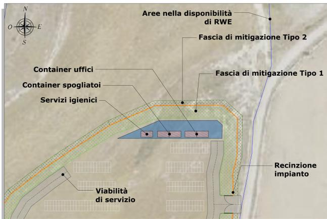
**DETTAGLIO 6 AREA DI CANTIERE - SCALA 1:500**
