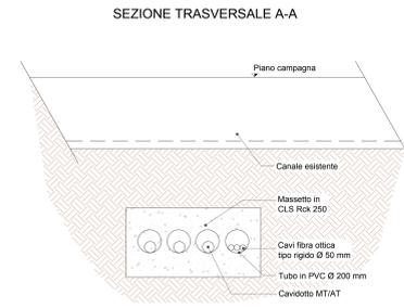
TIPICO DI POSA CON PROTEZIONE IN MASSETTO DI CLS (INTERFERENZA CON CAVI ELETTRICI) SCALA 1:20
