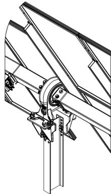
DETTAGLIO A :SUPPORTO MOTORE
