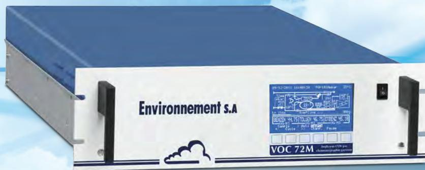
The VOC72M's metrology, **in accordance with EN 14662-3 standard** for benzene measurement, is based on gas chromatography (GC) for the separation of the measured compounds coupled with a photo-ionization detector (PID).
