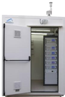
Example of fixed air quality monitoring station with rack version 2M series analyzers.
