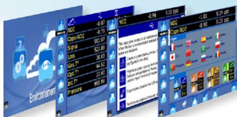
**NEW: on board web server and es@cloud™** user interface with on-line help for the display, configuration, maintenance, diagnostics or software updating of the analyser, remotely, from any PC, tablet or iPhone.
