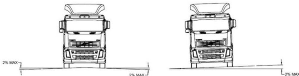
Figure 3 - Road cross-slope limitations
