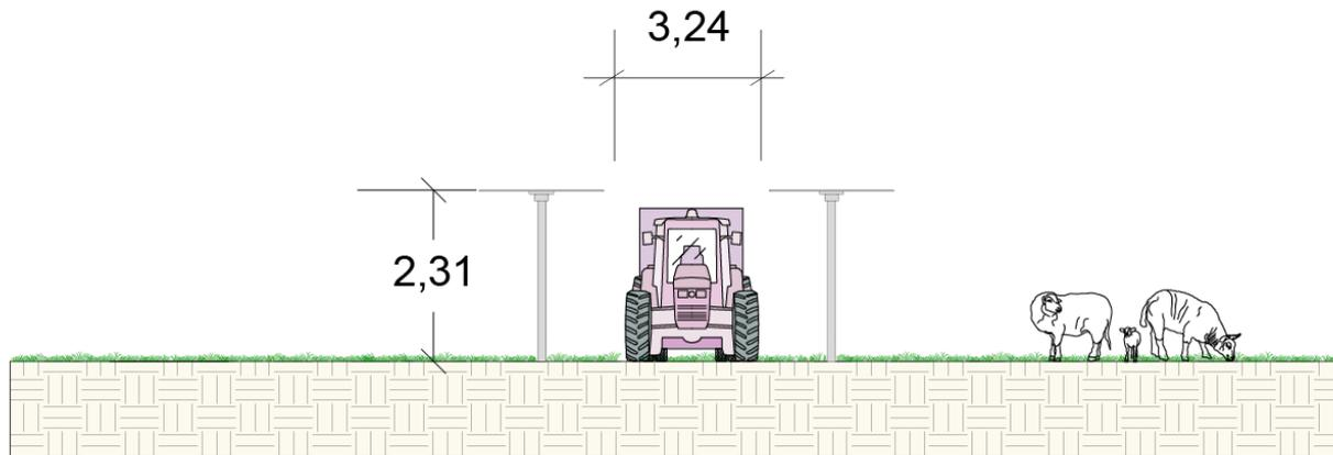
FIGURA 57 – SISTEMA AGRIVOLTAICO ELEVATO, SEZIONE TIPOLOGICA
