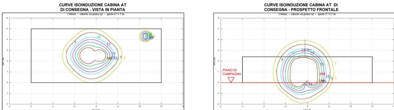
FIGURA 112 – CURVE ISOINDUZIONE CABINA AT CONSEGNA – PIANTA (A Sx) E PROSPETTO FRONTALE (A Dx). STRALCIO DELL'ELABORATO MRS-PDT13 E MRS2-PDT13.
