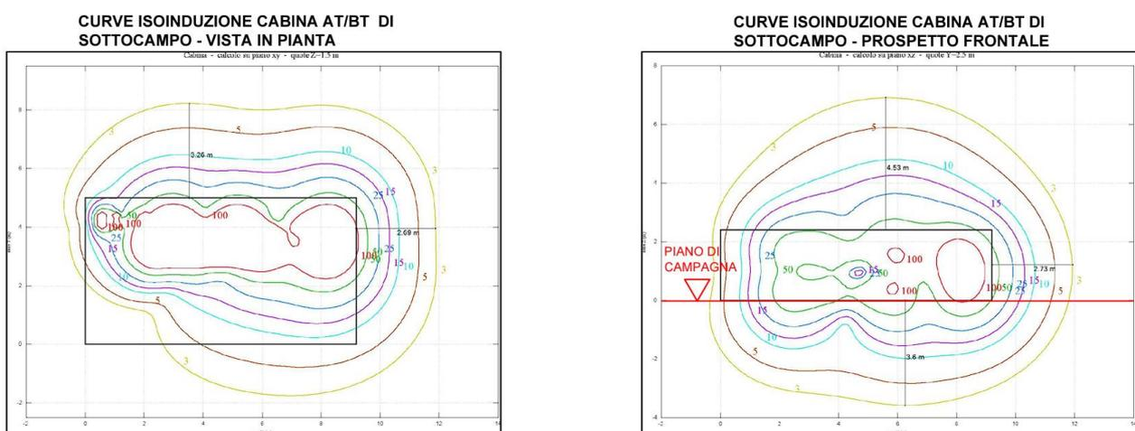
FIGURA 111 – CURVE ISOINDUZIONE AT/BT CABINA DI SOTTOCAMPO – VISTA IN PIANTA (A SX) E PROSPETTO (A DX). STRALCIO DELL'ELABORATO MRS-PDT13 E MRS2-PDT13
