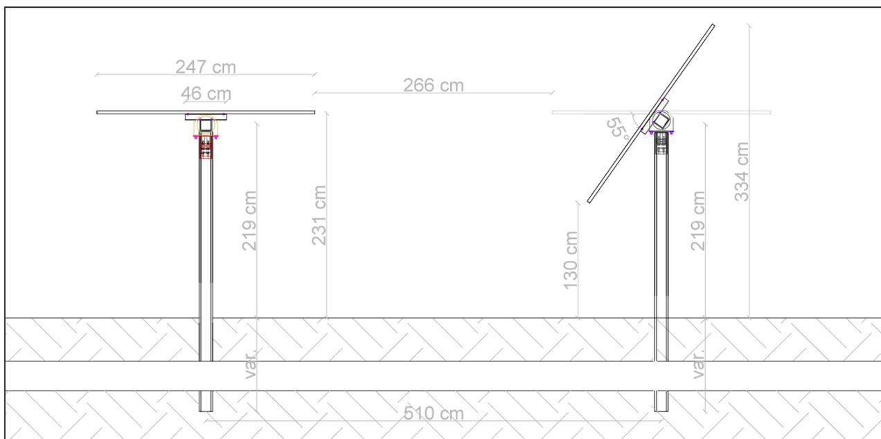
FIGURA 56 – TRACKER TIPO AD ASSE VARIABILE IN USO PER MORES 2 CON PITCH PARI A 5,1 METRI
