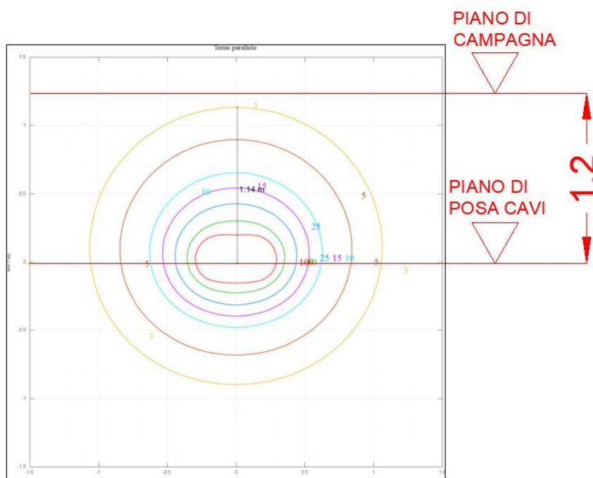
FIGURA 108 – CURVE ISOINDUZIONE – 3 LINEE BT INTERRATE INTERNE AL CAMPO FOTOVOLTAICO (STRALCIO MRS-PDT13 E MRS2-PDT13)
