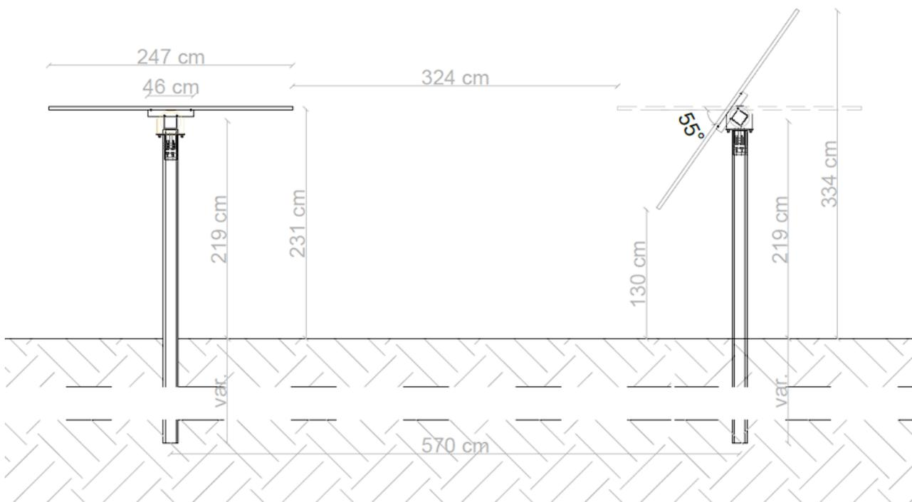
FIGURA 55 – TRACKER TIPO AD ASSE VARIABILE IN USO PER MORES CON PITCH PARI A 5,7 METRI
