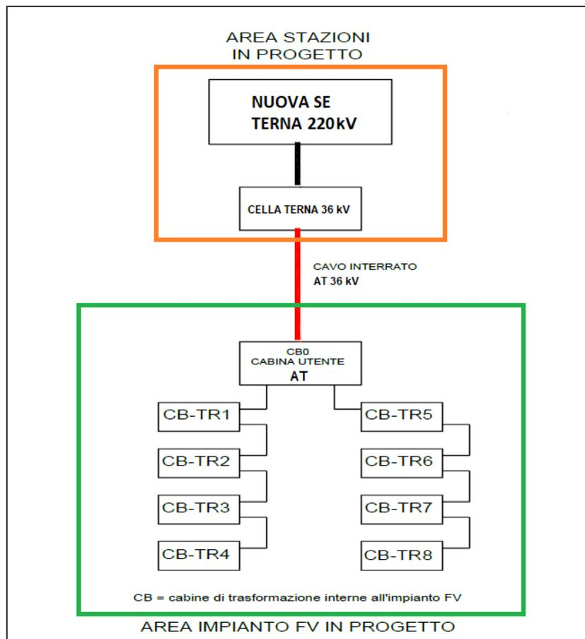
FIGURA 9: SCHEMA A BLOCCHI IMPIANTO
