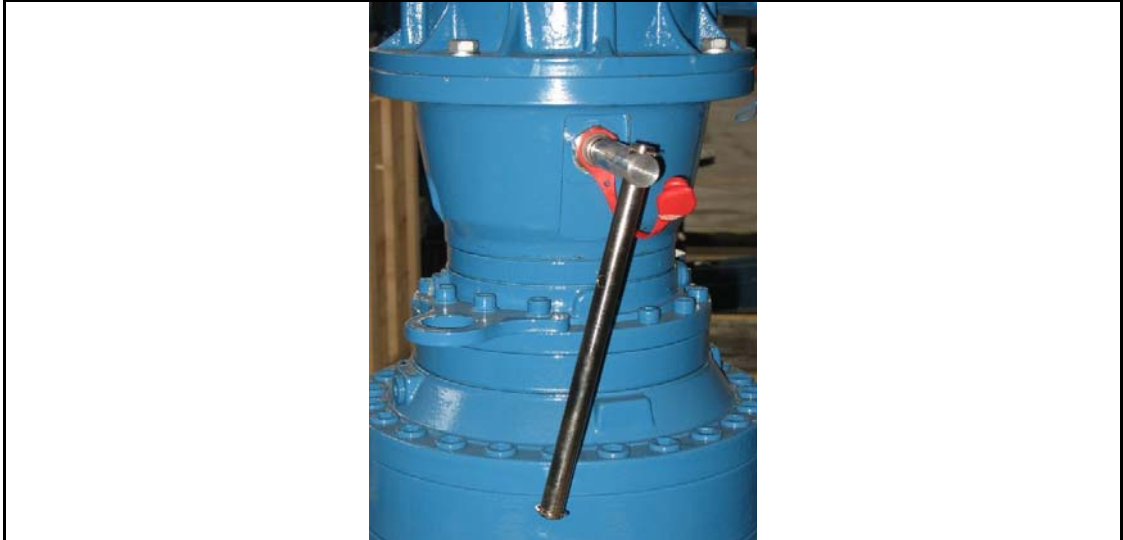
Fig. 22: Pitch locking device
