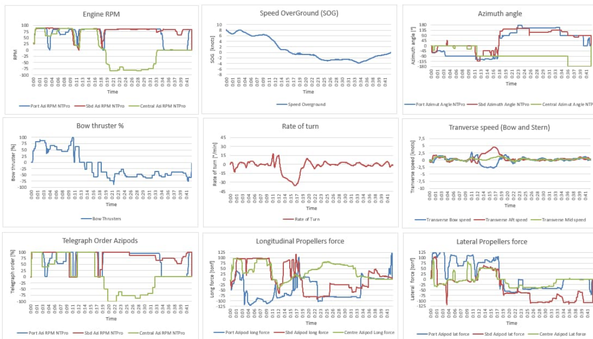
Figure 6.6: Exercise 4 swept path and time histories of main parameters of the Oasis vessel model
