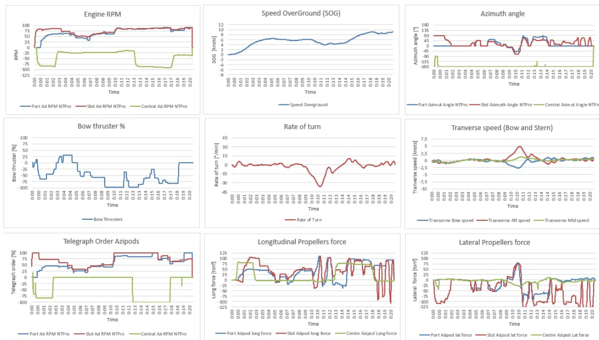
Figure 6.14: Exercise 12 swept path and time histories of main parameters of the Oasis vessel model
