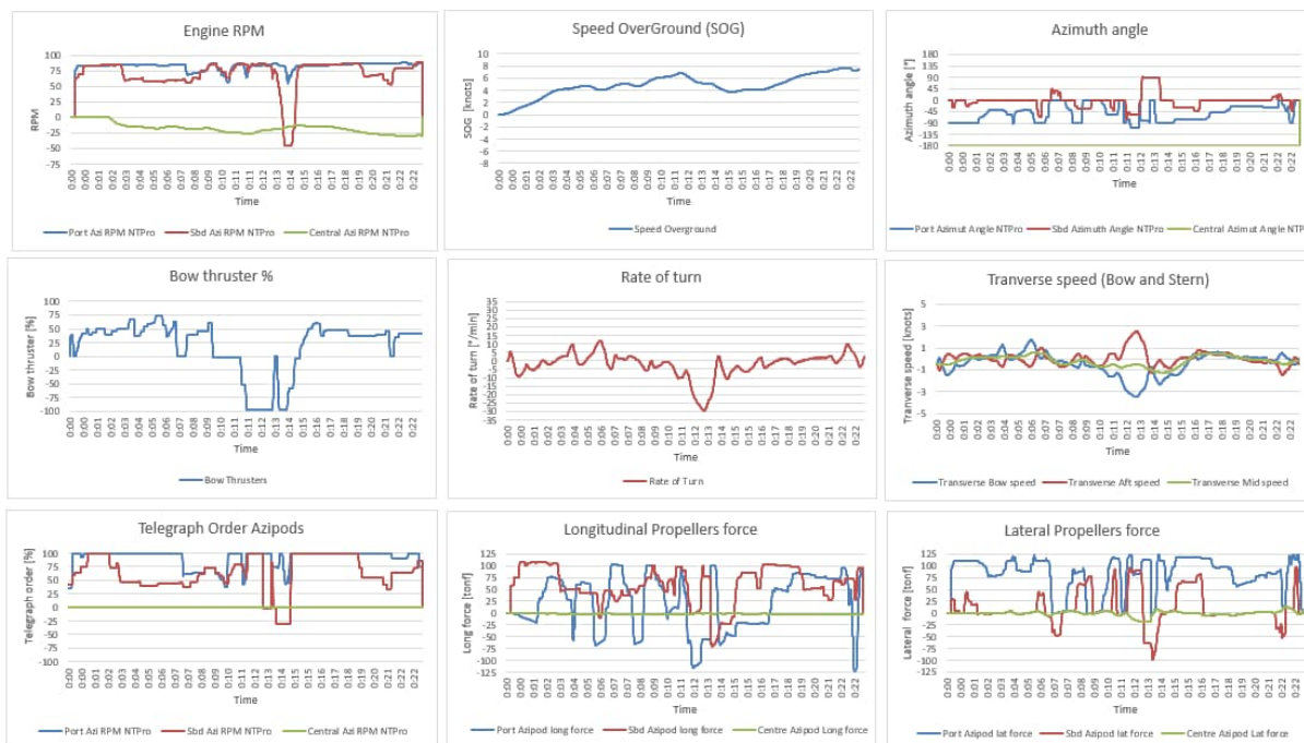
Figure 6.11: Exercise 9 swept path and time histories of main parameters of the Oasis vessel model
