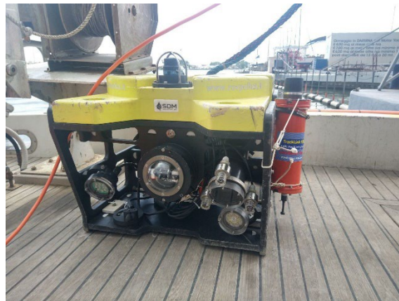
Figure 4.3: ROV Pollux III with TrackLink beacon.
