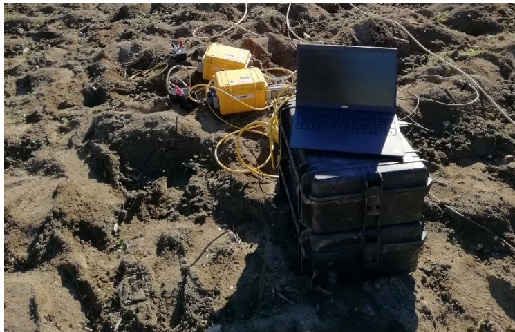
Figure 2.2: Seismograph GEOMETRICS "GEODE" and notebook
