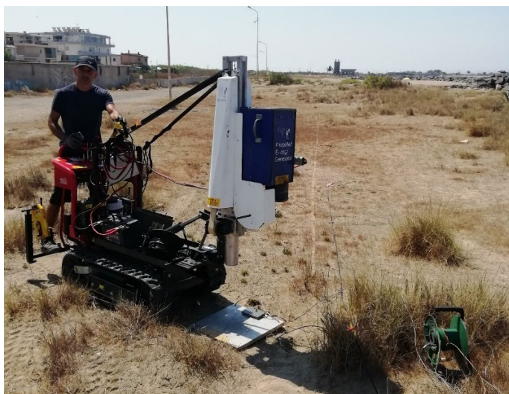
Figure 2.1: Energy source employed: accelerated weight on tracked vehicle.
