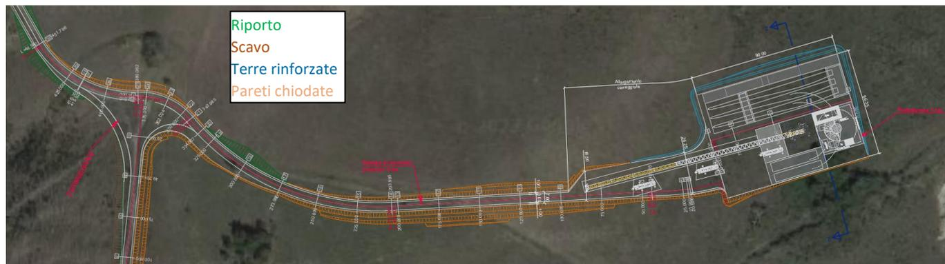
Figura 56: Pianta Layout piazzola WTG3
