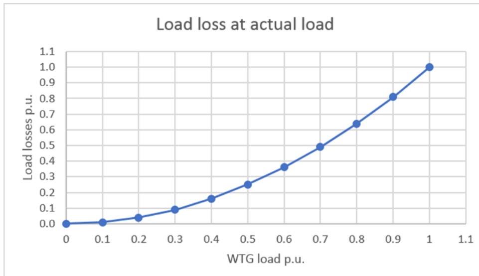
Figure 4-2: Transformer load losses scaling
