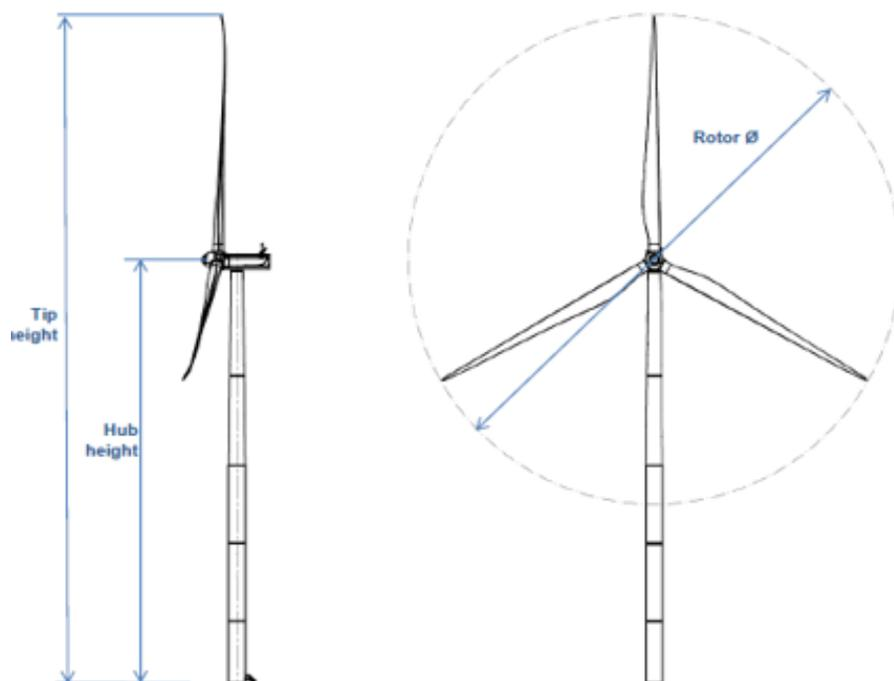
Tip height=200m; hub height=114m; rotor diameter=172m; blade length= 86m.
