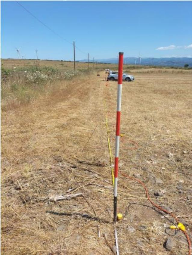
Sismica a Rifrazione/MASW R3-M3
