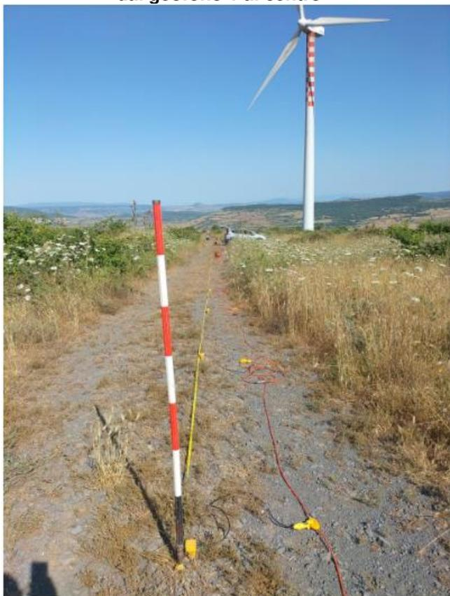
Sismica a Rifrazione/MASW R1-M1
