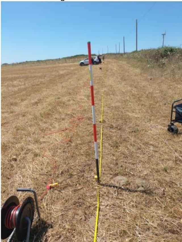
Sismica a Rifrazione/MASW R3-M3
