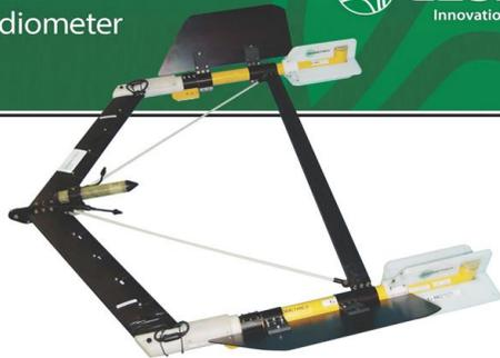
Geometrics' model G-882TVG Transverse Gradiometer system mates our proven, high-performance cesium sensor with dual high-sensitivity and high-speed CM 221™ Larmor Counters. This advanced integrated magnetometer system provides unmatched versatility in performance, with a 1.5m-wide sensor separation for maximum target detection efficiency and survey cost effectiveness.
