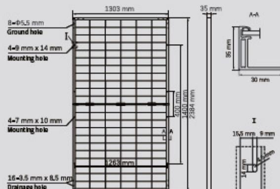
Figura 3 – Modulo agro-voltaico Astronergy TWINS CHSM66M(DG)/F-BH 655 W
