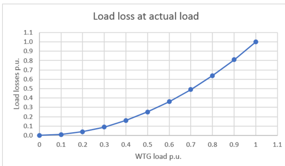
Figure 4-4: Transformer load losses scaling
