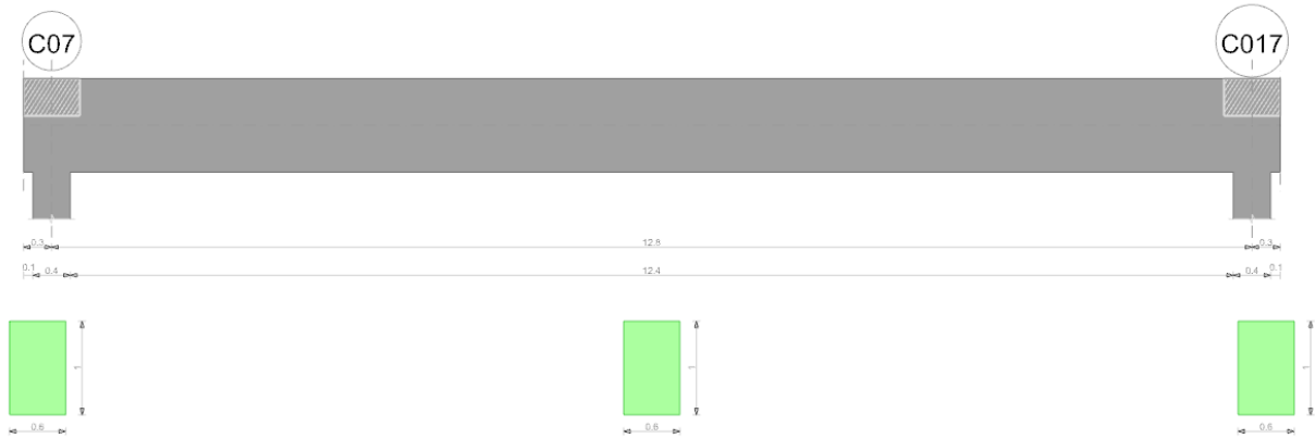
Fig. 62. Geometria travi 600x1000
