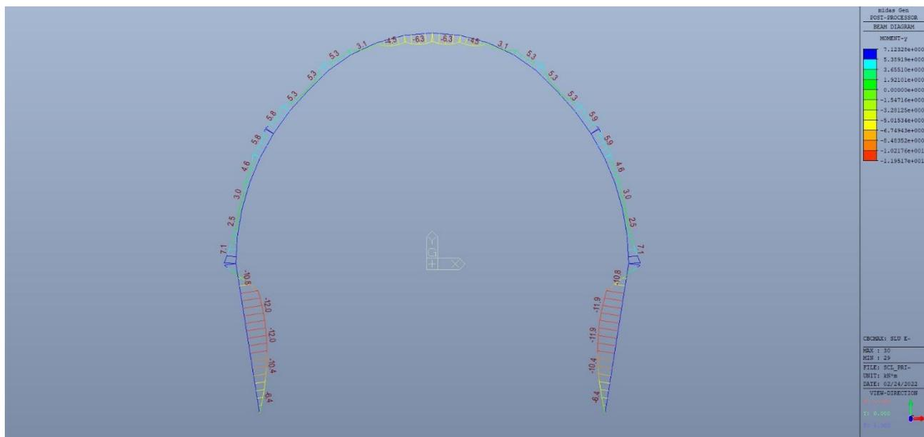
Fig. 4 – Envelope SLU Bending Moment – Prima Fase
