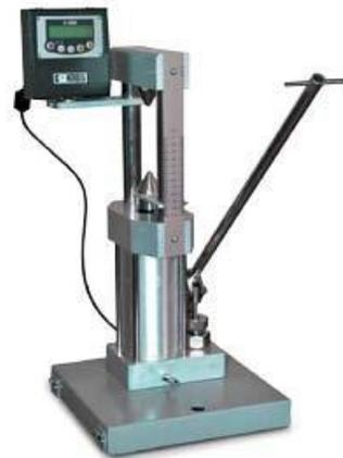
Fig. 12 – a) schmidt hammer b) Point Load Test
