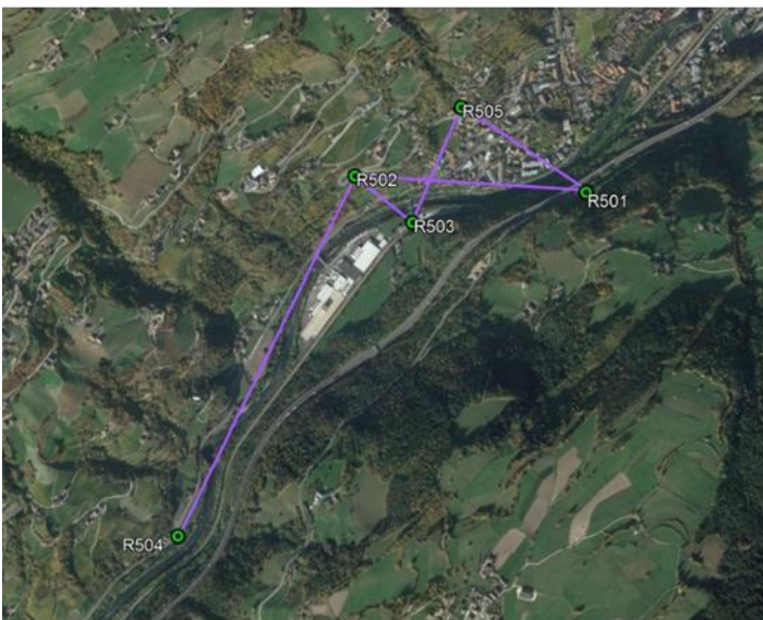
Fig.12 Rete Raffittimento R501 – R502 – R503 – R504 – R505
