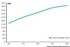
One wind turbine, 100% availability, 0% losses, k factor =2, Standard air density = 1.225, wind speed at hub height
