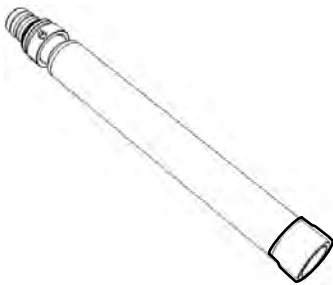
Figure 61 Turbidity sensor storage
