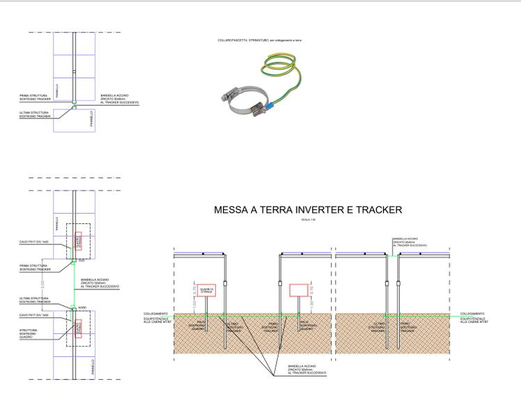
Collegamento a terra Inverter e Power Station
