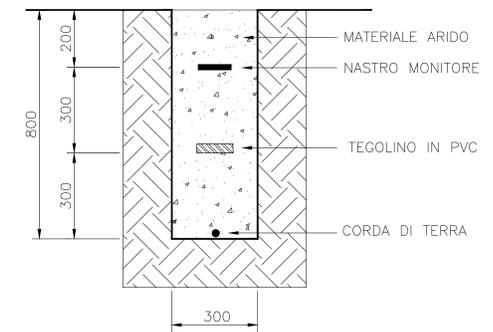
**SEZIONE SU STRADA STERRATA TIPO "MS" - TORRE METEOROLOGICA**
