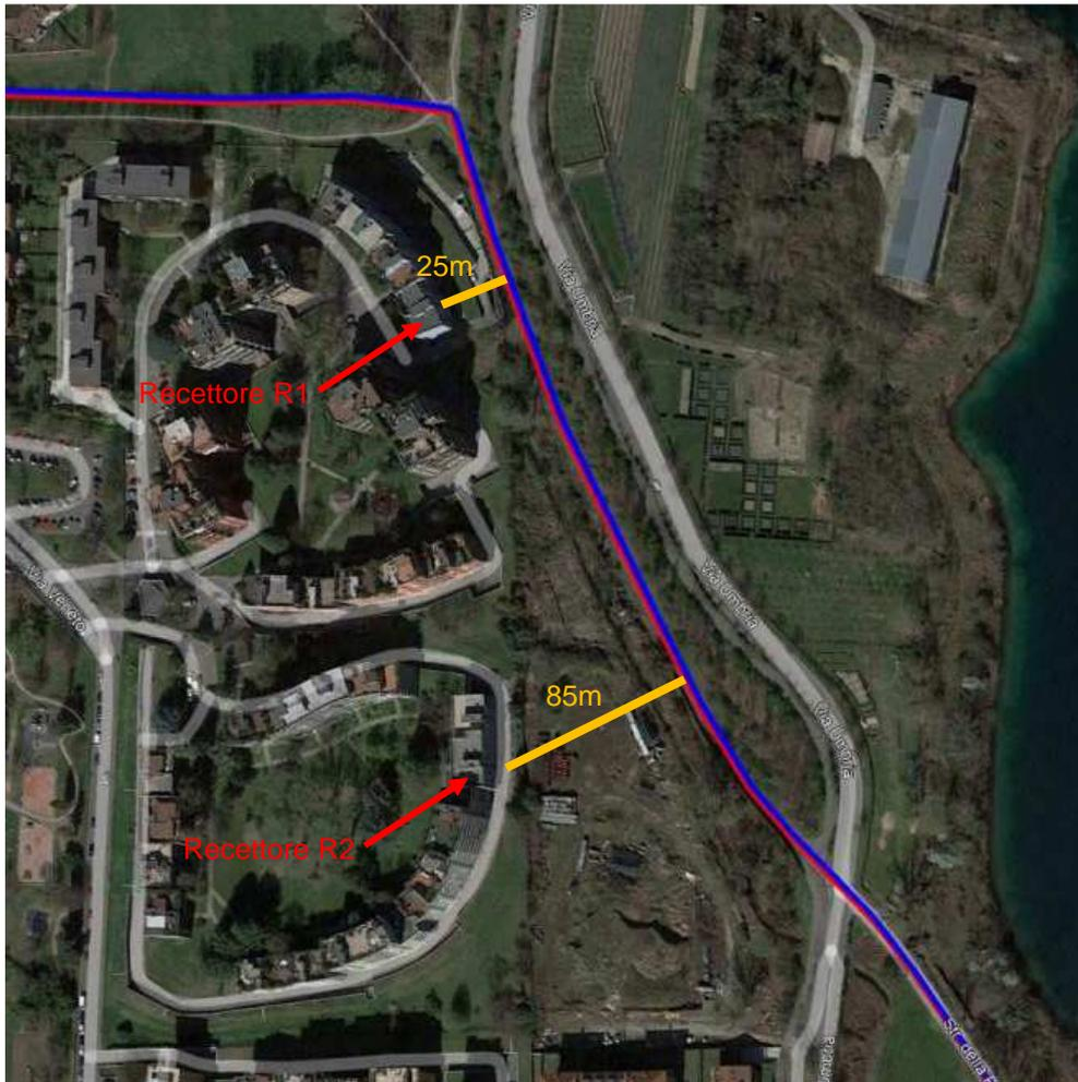
$$L_{P\_Fase1-R1} = L_{AW_{Fase1}} - 20\log(25m) - 8 = 108.5 - 20\log(25m) - 8 = 72.5 \text{ dB(A)} > 55 \text{ dB(A)} \text{ Classe III}$$
