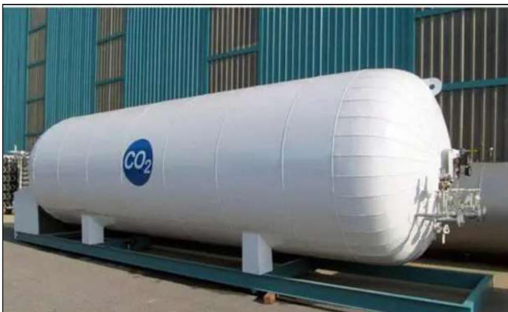
FIGURA 3-32: STOCCAGGIO CRIOGENICO DELLA CO<sub>2</sub> (VOLUME 50 M<sup>3</sup>)
