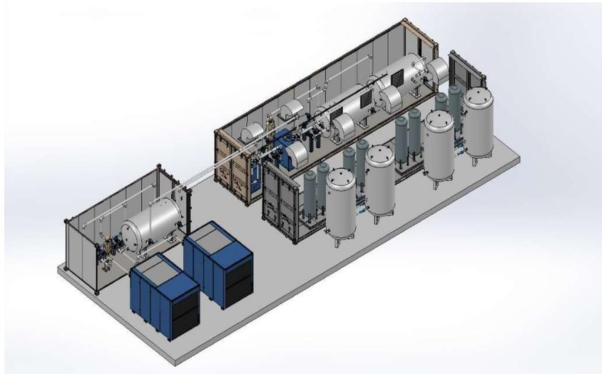
FIGURA 3-21: UNITÀ ARIA COMPRESA (UNITÀ 500 – PK-501 A/B/C, V-501, S-502) E UNITÀ DI GENERAZIONE AZOTO (S-601 A, S-601 B, V-602)
