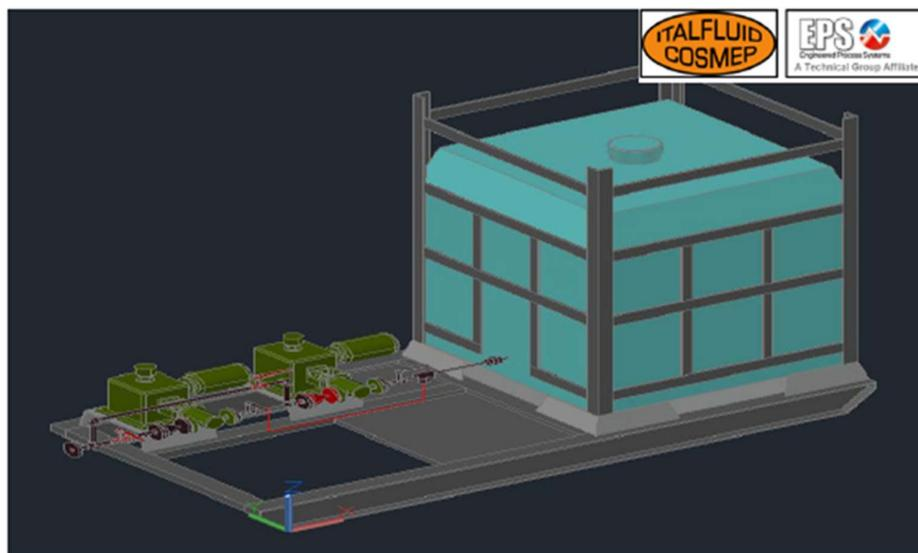
FIGURA 3-3: PACKAGE INIEZIONE INIBITORE DI CORROSIONE CI-190-A
