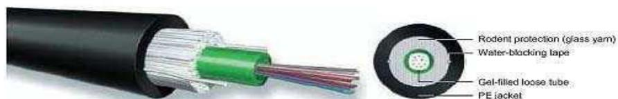
Figure 1: Fibre optic cable (cross section)
