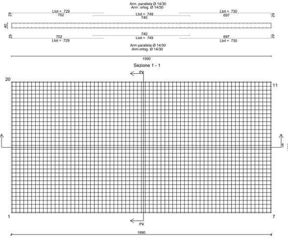
**ARMATURA DI BASE INF.=SUP. PIASTRA DI BASE QUOTA m.0.00**
