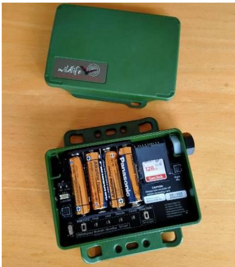
Figura 2.4/C. Bat detector Song Meter Mini Bat Ultrasonic recorder della Wildlife Acoustics
