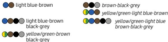
Conductors for signalling cables are black, with numbers and with yellow/green earth conductor
