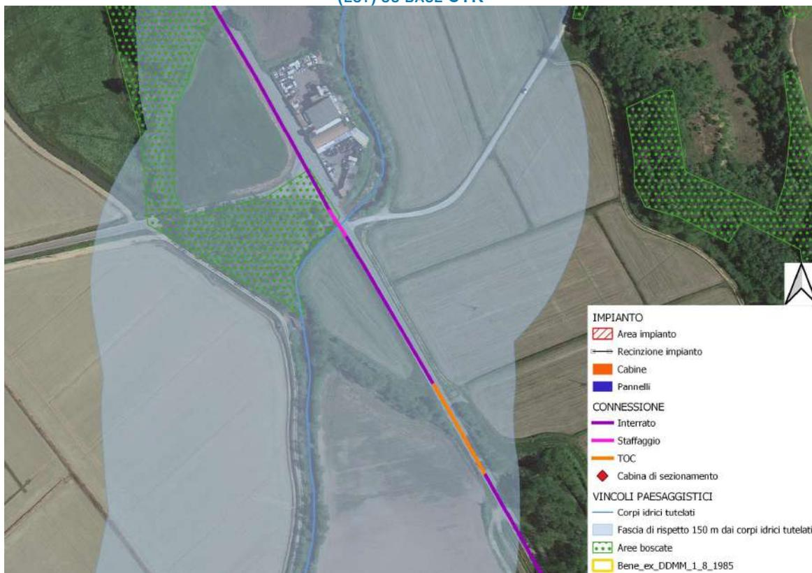
**TRATTO DI CONNESSIONE INTERFERENTE CON LA FASCIA DI RISPETTO DEL RIO GUARABIONE. IL PRIMO TRATTO (IN ROSA) AVVERRÀ TRAMITE STAFFAGGIO AL PONTE, IL SECONDO AVVERRÀ CON SCAVO TELEGUIDATO IN SUBALVEO, SU BASE ORTOFOTO**
