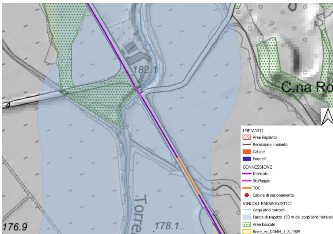
**TRATTO DI CONNESSIONE INTERFERENTE CON LA FASCIA DI RISPETTO DEL RIO GUARABIONE. IL PRIMO TRATTO (IN ROSA) AVVERRÀ TRAMITE STAFFAGGIO AL PONTE, IL SECONDO AVVERRÀ CON SCAVO TELEGUIDATO IN SUBALVEO, SU BASE CTR**
