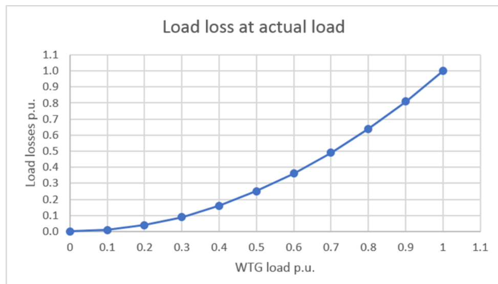
Figure 4-4: Transformer load losses scaling
