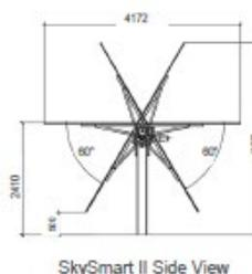
**Fig. 8 - Datasheet tracker SkySmart II (ARCTECH)**
