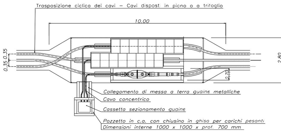
**CASSETTA DI SEZIONAMENTO PER CROSSBONDING**
