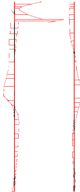
Fig. 11 Shear forces envelop in beam Extreme value -1,04 \cdot 10^3 kN/m (Phase: 8)
