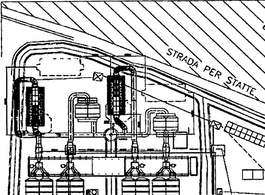
PWDE drawing: 153101816-30200-10 (showing step 3; installation of last two new bag filter plants)
